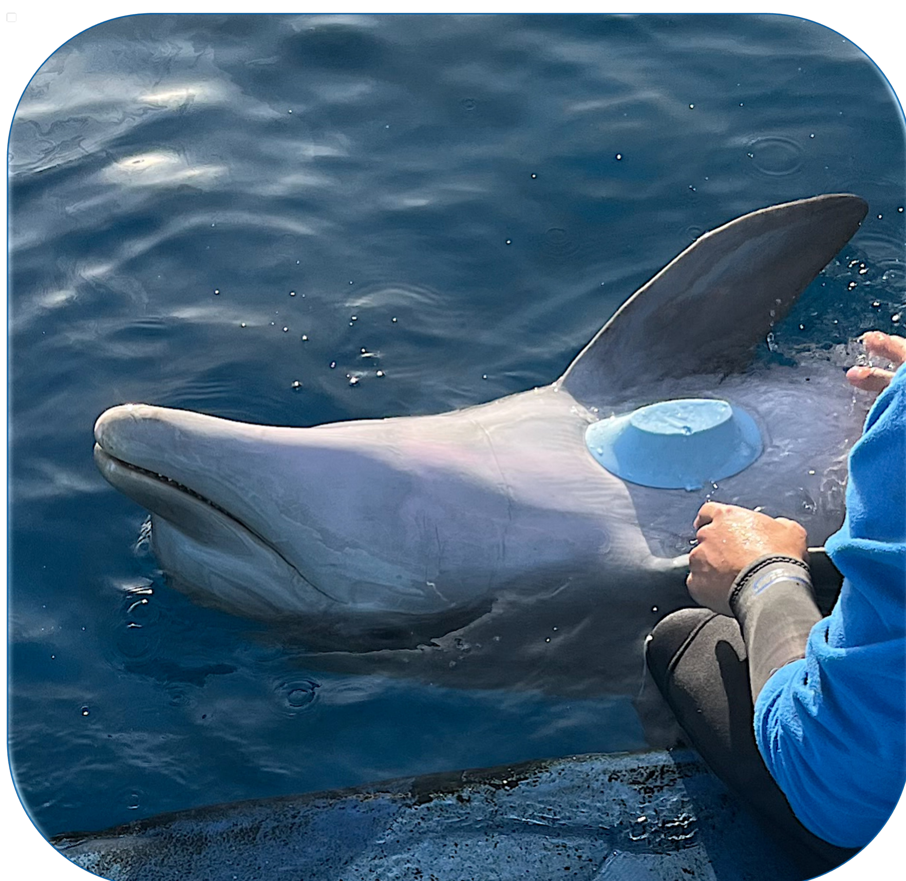
Figure 1. ECG physio-logger incorporated in a single suction cup attached to the sternum of a dolphin.
