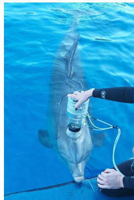
A custom-made pneumotachometer was used to sample breathing for 5-7 minutes
