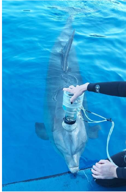
Figure 2. A custom- made pneumotach was used to sample breathing
