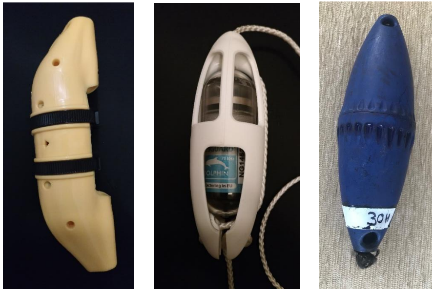
Figure 1. Pictures of the pingers in their casings. The Banana pinger from Fishtek (left), the Netguard Dolphin Pinger from Future Oceans (center) and the PAL pinger (right).
