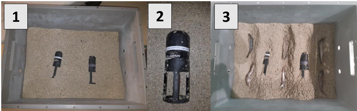
Figure 6 Pictures of the organisation of the shell sand box with the two sonar targets inside. 1) The positioning of the two targets in the box. 2) Close up of the sonar target. 3) The positioning of the fish in the box.
