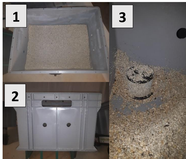
Figure 5 Close-up of one of the shell sand boxes. 1) Top-down view. 2) Short side view. 3) Close up of the filter covering the drainage hole.
